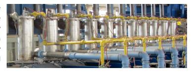
**★ Excellent Bath Temperature Uniformity** — The immersion tube high heat-transfer rate promotes a convective "stirring" in the bath that distributes the zinc temperature evenly. The convective currents also keep much of the Zn-Fe in suspension, considerably reducing dross accumulation in baths with heavy coat production.
