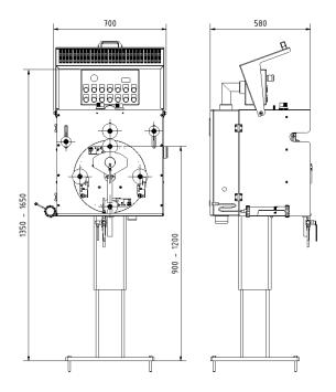
The CP 4R is an automatic cable printing machine with electronically controlled printwheel drive and automatic printwheel changer. This type of drive allows printing at speeds of up to 1500 m/min.
